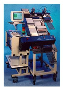
Early field trials of predecessors to Exatron's newest Model 5000 handlers - designed and engineered to meet heavy-duty production handling requirements - uncovered a problem that needed guick correction: 6061T6 aluminum trackwork on the company's pioneering handlers was subjected to potentially damaging ESD (Electro-Static Discharge) caused by the constant movement of plastic and ceramic leaded integrated circuits sliding down the 6061T6 aluminum
