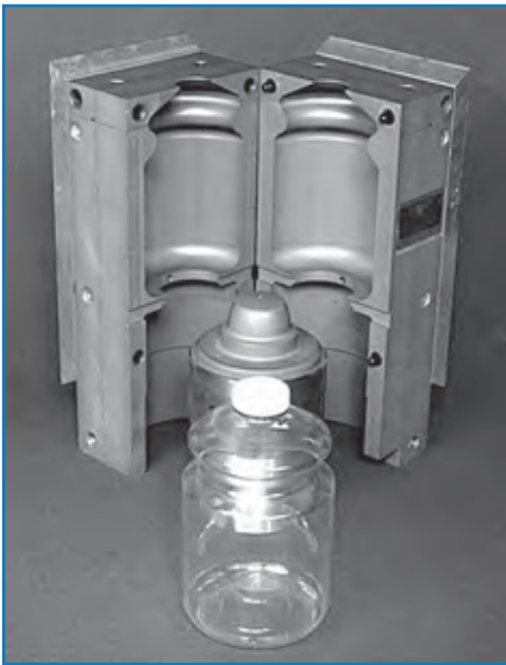
TUFRAM on aluminum sections of Johnson Controls' bi-metallic PET bottle molds prevent erosion and galvanic corrosion causing poor release, high reject rates and shortened mold life. Steel sections are treated with Magnaplate's NEDOX®.
