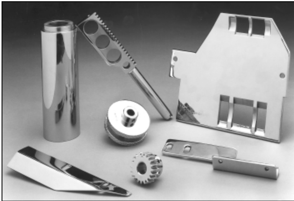
Cigarette-making machine parts are coated to eliminate scratching of film and package.
