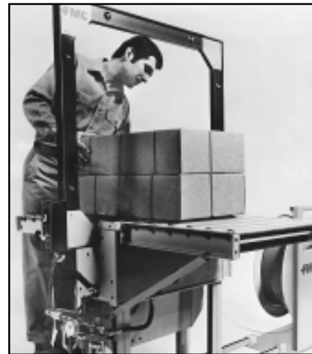
Aluminum yoke and a variety of steel components on FMC's high-volume strapping machine are protected against abrasive wear by Magnaplate "synergistic" dry-lubricated coatings.
