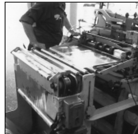
Side folding plates (left) and bottom fold plates (right) on the over-wrap machines used to wrap Marcal Paper's pocket tissue packs have been protected with Magnaplate HCR® to resist wear and reduce down time.
