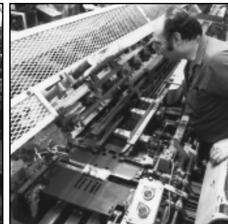
Side folding plates (left) and bottom fold plates (right) on the over-wrap machines used to wrap Marcal Paper's pocket tissue packs have been protected with Magnaplate HCR® to resist wear and reduce down time.
