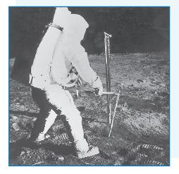
CANADIZE treatment on both the inside and outside of the Titanium core-sample drill tubes used in NASA's exploration of the moon's surface prevented galling at the joints and in the drive shaft. It also eliminated the danger of contamination of moon rocks samples by titanium particles or other foreign materials.
